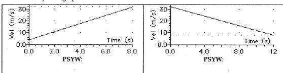
The area under the line of a velocity-time graph can be calculated using simple rectangle and triangle equations. The graphs below are examples:
