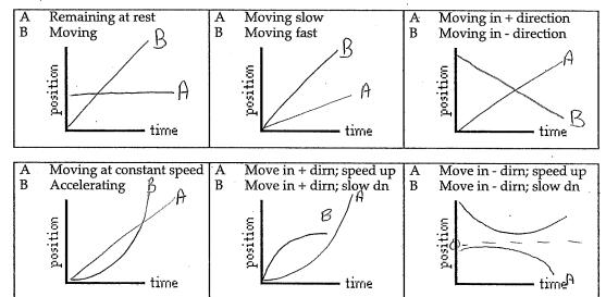
3. For each type of accelerated motion, construct the appropriate shape of a position-time graph.
